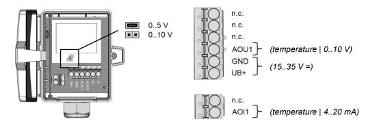
AKF10+ (LCD) TRV MultiRange Relay
