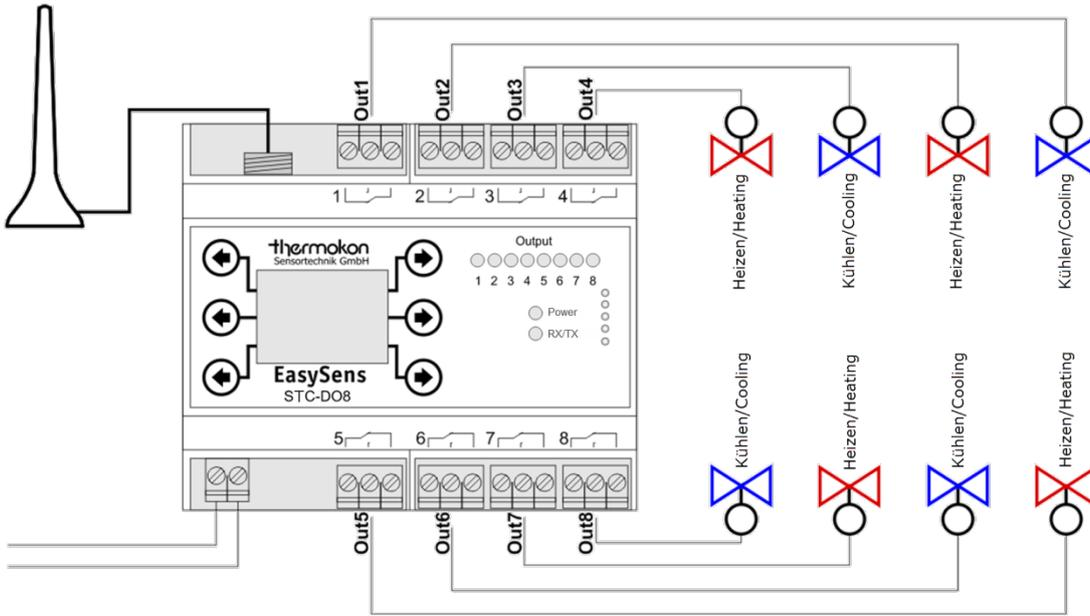
Heating / cooling with combined heat-/cooling valve (2-pipe system)
