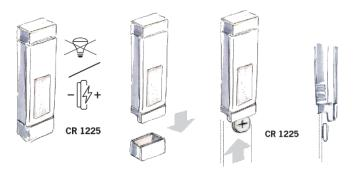
If the sensor is installed in a location where the light intensity is constantly too low, a button cell can be used to supplement the harvester. Use only CR1225 button cells.
